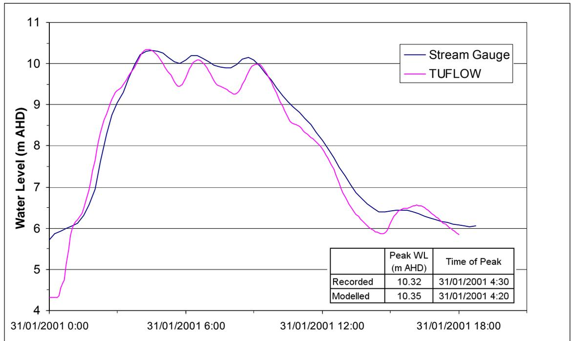
The TUFLOW model produced a peak flood level 30mm higher than the recorded flood level at the Sackville Street stream gauge, suggesting a good combined calibration of the XP-RAFTS and TUFLOW models. Typically calibration to within 100mm of the recorded peak water levels would be considered satisfactory. As mentioned previously, the XP-RAFTS model was not calibrated separately, and the flows were routed hydraulically in TUFLOW.
