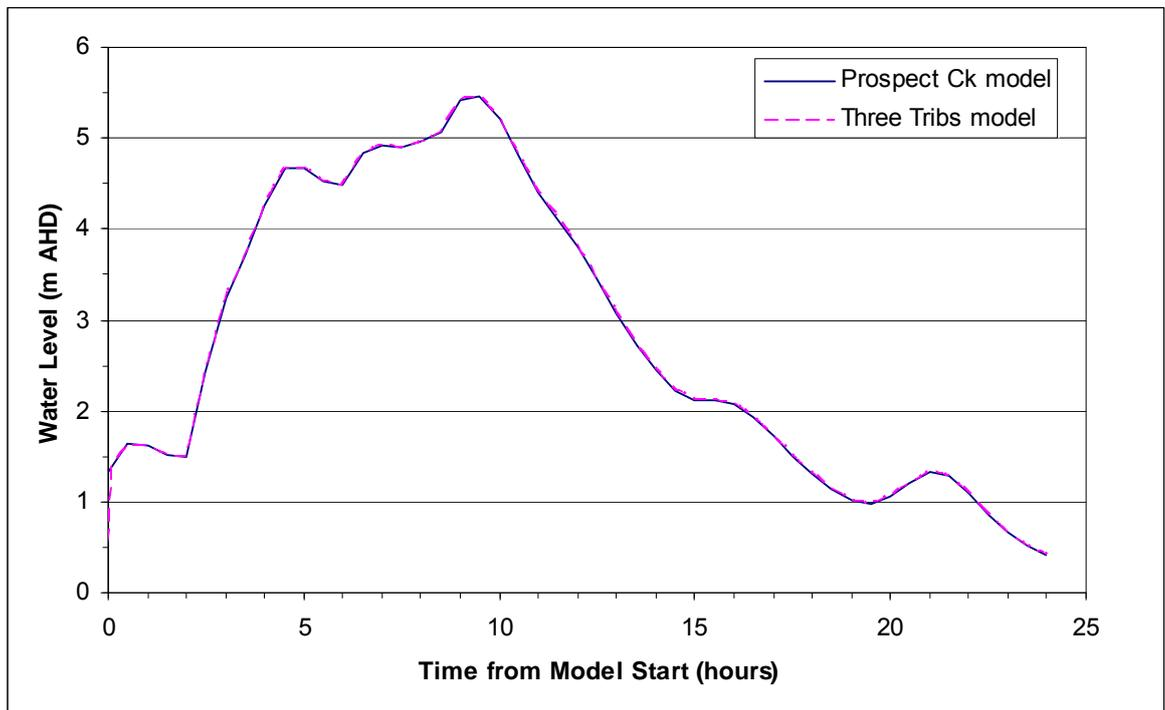
■ **Figure 4-7 Modelled 2001 event stage hydrographs, downstream of railway bridge**
