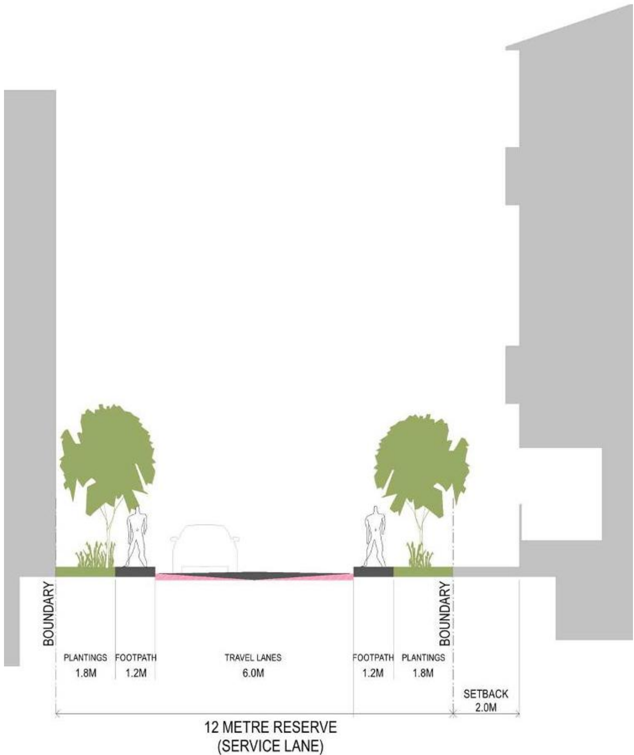
Figure 6: Service lane, 12m reserve Note: Building profiles and heights are indicative only
