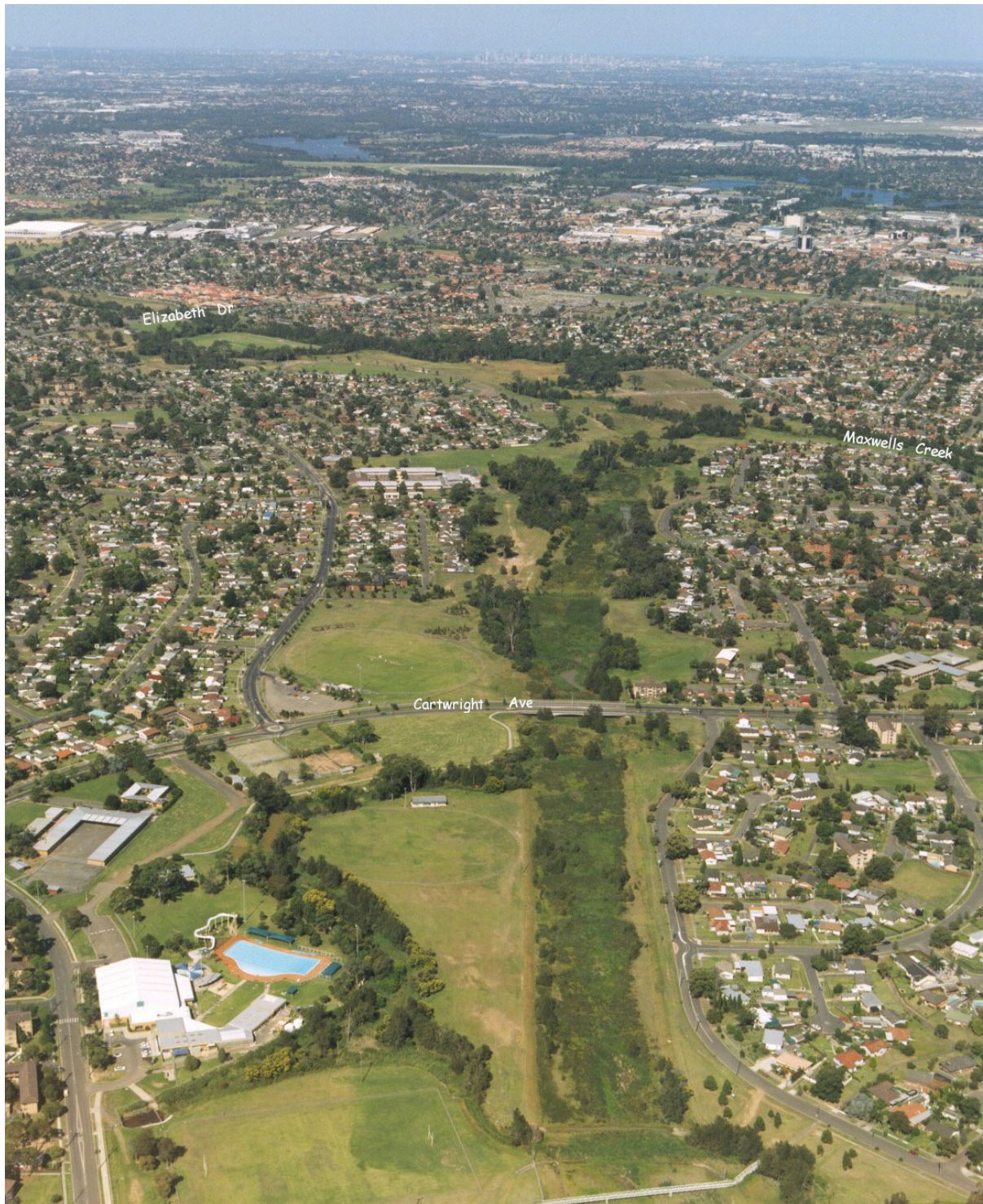
Oblique aerial photo of Lower Cabramatta Creek (November 1998), viewed from the middle of the catchment downstream to the Georges River. Most of the lower floodplain is located within open space reserves. A formed floodway that was constructed some 30 years ago is prominent in the foreground.
