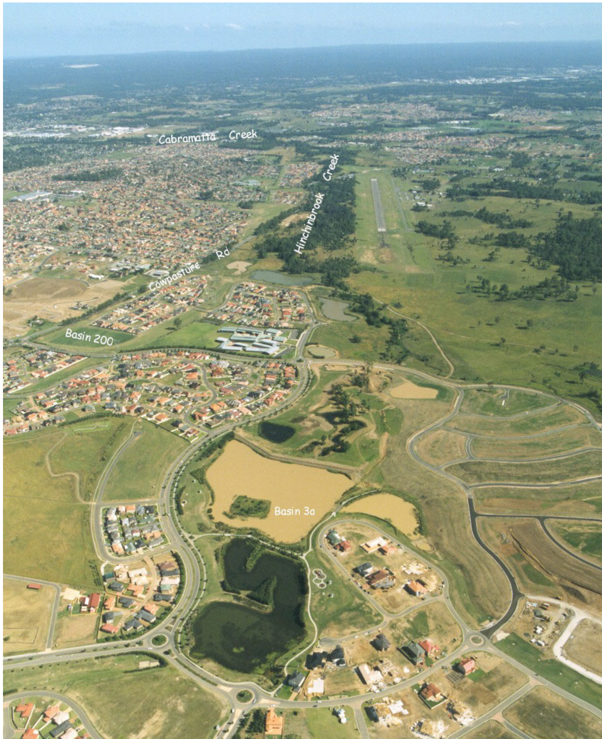
Oblique aerial photo of Hinchinbrook Creek (November 1998), viewed looking downstream towards Cabramatta Creek. New release area development in Cecil Hills is evident, along with compensatory detention basins and smaller water quality basins.
