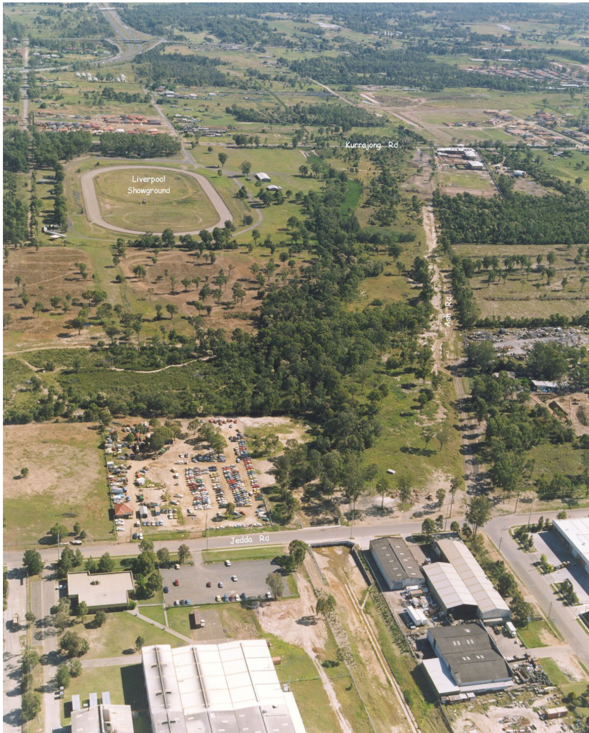
Oblique aerial photo of Maxwells Creek (November 1998), viewed from Jedda Road upstream towards Camden Valley Way. Downstream of Jedda Road the creek consists of a formed channel with concrete invert. The creek reverts to a more natural form between Jedda Road and Kurrajong Road.
