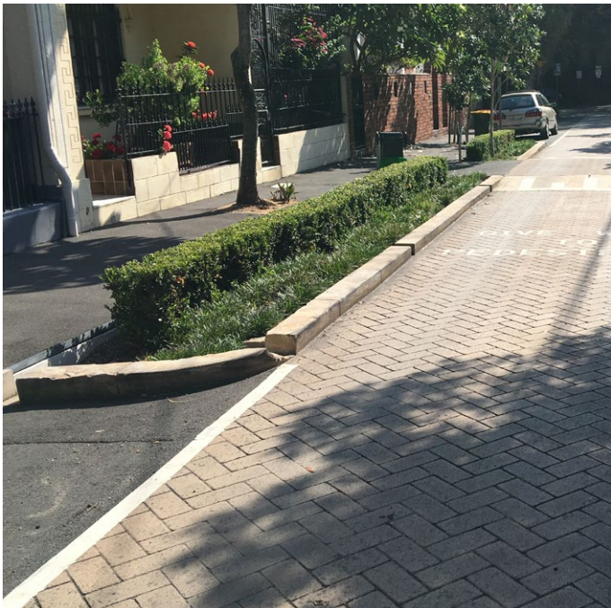
Traffic calming measures can be designed to accommodate parking include planting and improve the quality of the public domain
