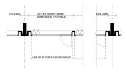
Figure 14A - Awning type B - Internal awning plan
