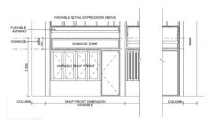
Figure 14B - Awning type B - Shopfront and awning elevations
